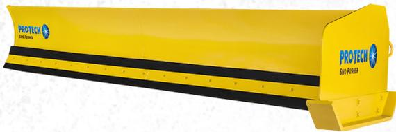
Clear snow from underneath parked trailers, especially the fifth wheel pins. The Low Profile is 30” tall and 18’ wide. Its offset design allows for 6’ of reach under obstacles and windrows snow to the side.
