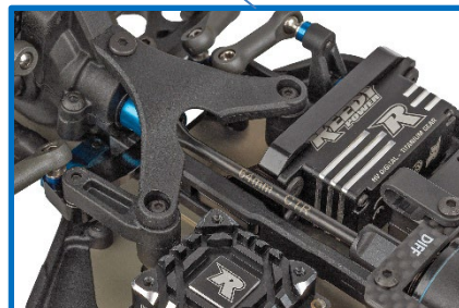
V2 Steering Posts and Bellcranks to Reduce Vertical Movement in the Steering Rack
