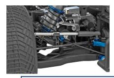
New truck specific gull wing long arm suspension. Includes anti-roll bars front and rear, accessible design based on RC10B7
