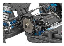
New 3-Gear Laydown Transmission
