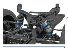
New front tower with hinged front bumper pivot and SC7 adjustable body mount system
