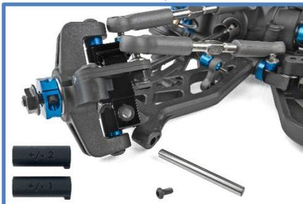
**Insert adjustable caster block with 0, +/-1, and +/-2 degree inserts included**
