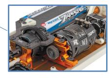
Forward and Back Motor Positions: used for further weight bias adjustment
