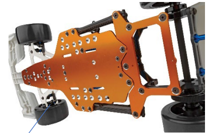
Machined countersunk Aluminum Gold Chassis and lower bracket
