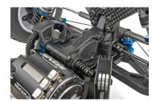
New 3-Gear laydown transmission
