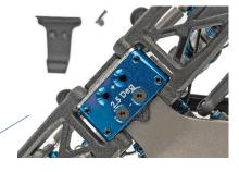
New truck specific gull wing long arm suspension with low CG truck shocks
