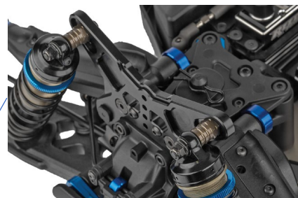
Includes FT hard-anodized aluminum shock bushings
