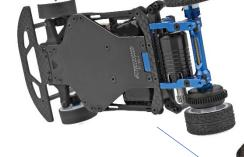
Steel chassis plate for low center of gravity
