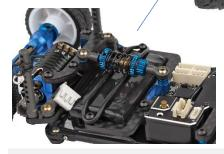
Easily removable battery holder to access the battery without removing center shock
