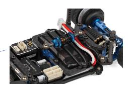
Threaded aluminum center shock with adjustable droop and spring collar
