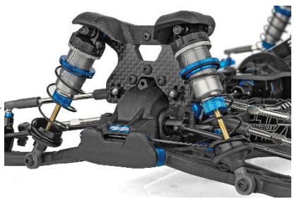
25mm and 31mm Length 13mm Big-bore Shock Bodies
