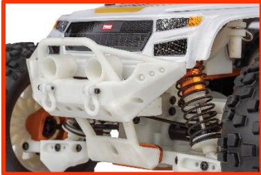
Durable, impact-absorbing front bumper with LED mounts
