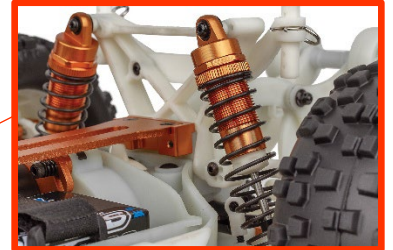
Threaded, Aluminum, Gold, oil-filled, coil over shock absorbers
