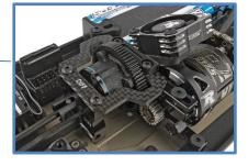
Forward and Back Motor Positions: used for further weight bias adjustment
