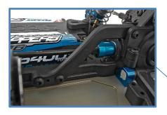
**Chassis Bracing:** fine tune chassis flex characteristics with upper and lower chassis bracing front and rear
