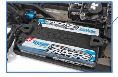
**Highly Adjustable Battery Holder with Thumb Tabs:** allows for easy battery removal and fine tuning of weight bias
