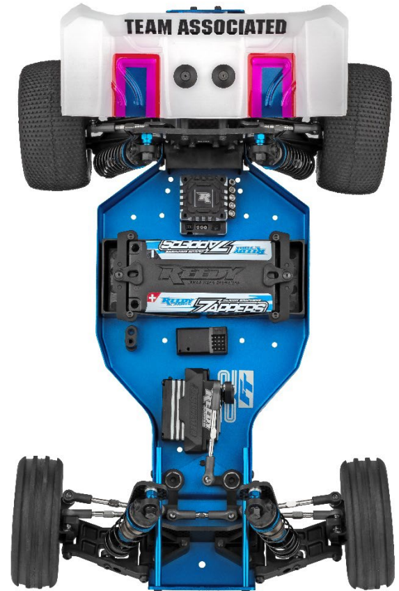
Rear shock tower integrates B6 rear wing mount
