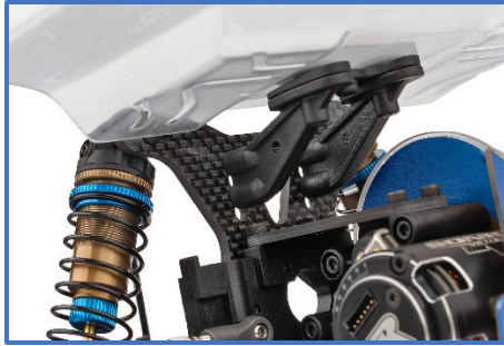
Rear shock tower integrates B6 rear wing mount
