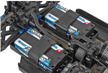
Adjustable battery tray design with hook and loop strap for retaining batteries
