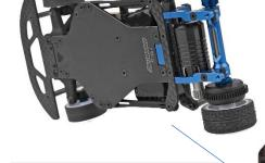
Steel chassis plate for low center of gravity
