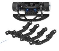
Fixed arm style front end with optional molded upper arms to adjust caster and camber
