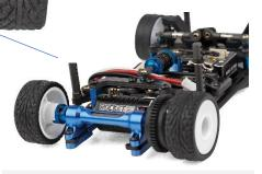
Two-piece rear pod with adjustable axle heights for different tire diameters and ride heights utilizing Factory Team carbon fiber shims
