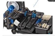
Easily removable battery holder to access the battery without removing center shock
