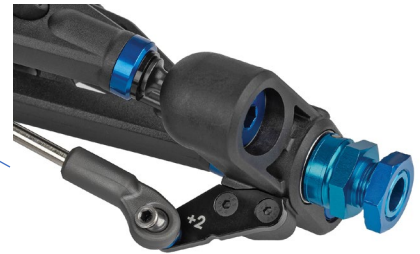
New 16deg KPI steering block with updated bump steer geometry
