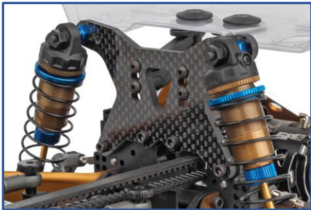
New rear Carbon Fiber shock tower integrates B6 wing mount
