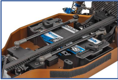
Bronze anodized 6061-T6 aluminum monocoque 4wd tub chassis
