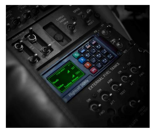
data and tracking functions from multiple remote locations in the aircraft. It is frequently installed in the aircraft cabin by air medical operators, which mainly allows air medics to communicate directly with ground personnel. This bypasses the need for communications to go through the flight crew, a significant benefit where time is paramount in providing patients with the best care possible.
